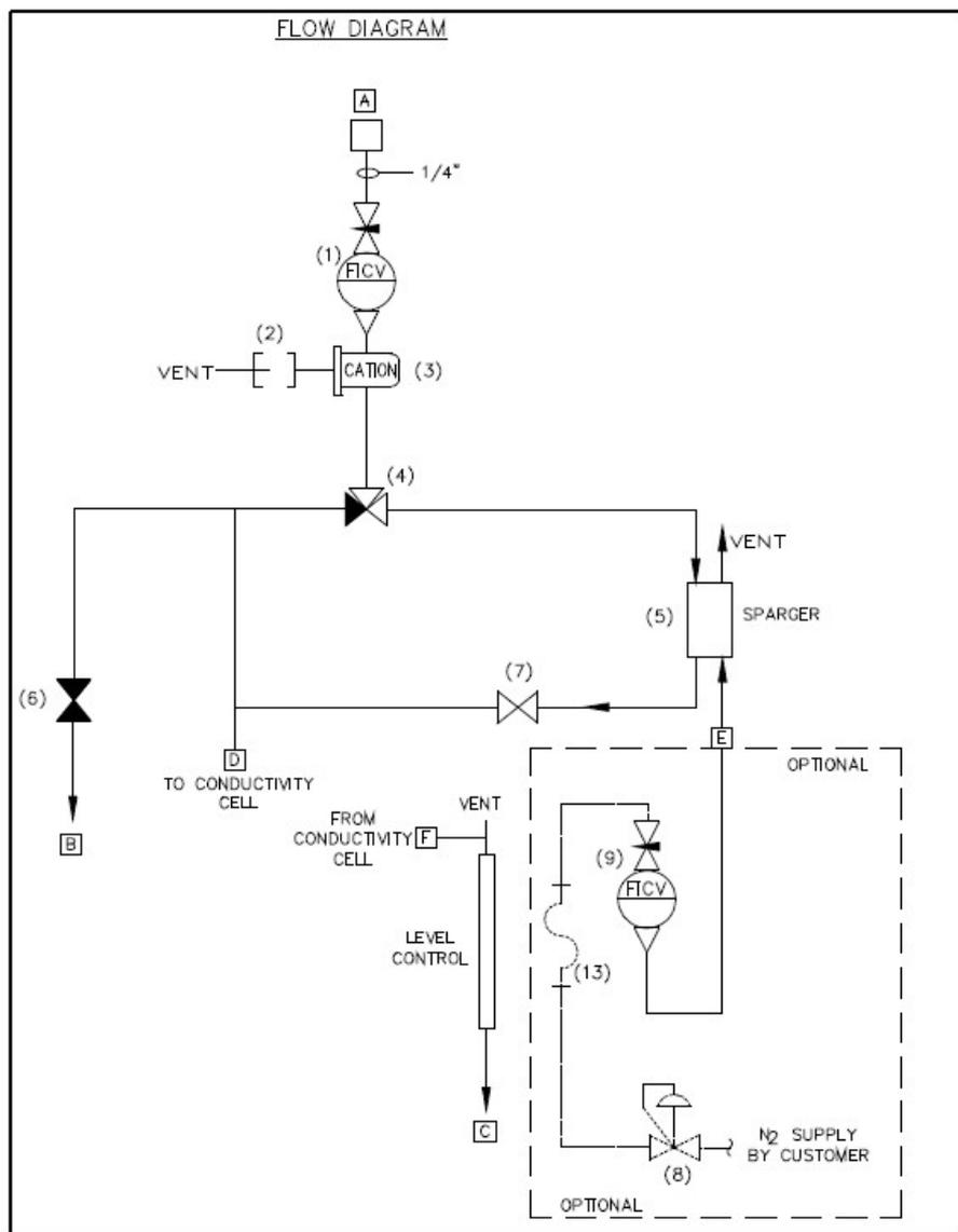
A typical flow diagram is shown above. The sample enters at the top, through a valved sample flowmeter, and then through the cation resin column.
