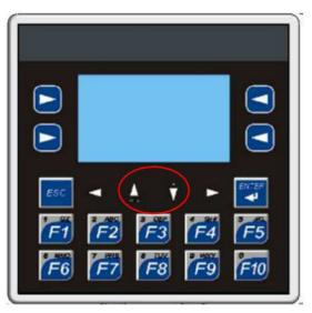
**3.** Once in the system menu locate Removable Media using the down arrow on the PLC. Press enter to open the Removable Media Manager in the System Menu and press the F4 (key 4) function key. After selecting Ok the application will be saved in a file called DEFAULT.PGM in the Micro SD root directory.
