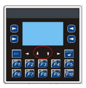
**3.** Once in the system menu locate Removable Media using the down arrow on the PLC. Press enter to open the Removable Media Manager in the System Menu. Find and highlight the desired .PGM file, and then press Enter.
