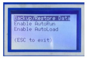
**4.** Hit F1 key (key 1) and create new back up by pressing enter, to backup data and registers. To restore data and registers press F2 (key 2) and hit enter which will reset the system.
